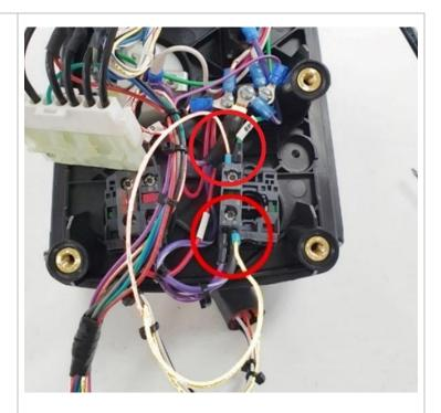
8. Connect the 8-pin connector from the operator sensor, and the 12-pin connector from the harness into the ECU.
