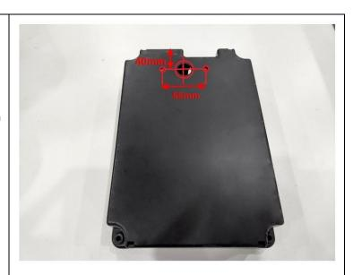
Drill two 5mm holes spaced
