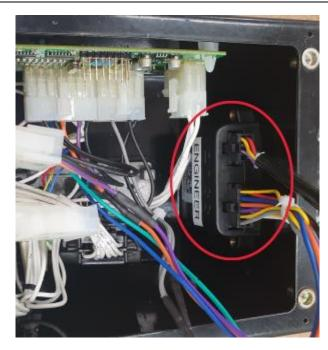
8. Route the operator sensor cable as shown in the image and secure the cable using cable ties.
