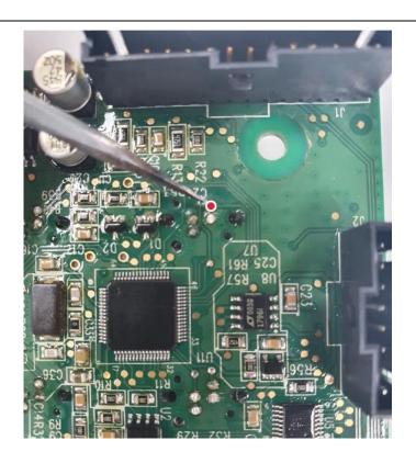
6. Behind the **Horn** push button, clean and expose the highlighted pins.
