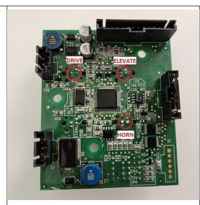
4. Behind the **Drive** select push button, clean, and expose the highlighted pins.
