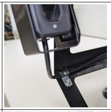
6 Operator sensor installation complete
