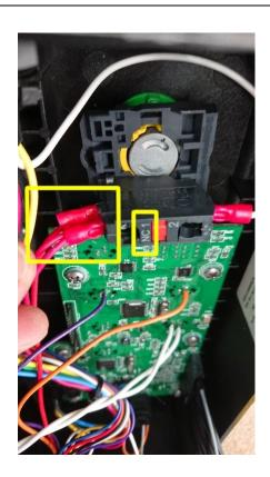
9. Using a hot glue gun, cover the exposed areas around the solder connections for the purple, orange, and white wires.
