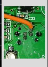
7. Remove the PCB coating around the two "HORN" pins highlighted in white with a sharp object to allow solder to flow.
