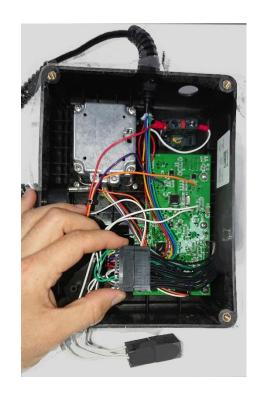
5. Remove the PCB coating around the "DRIVE" pin highlighted in white with a sharp object to allow solder to flow.
