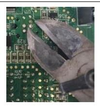
6. Trim down the **Elevate** signal pin. This pin is located as displayed in the image. Using a fine pair of side cutters make sure that the pin is trimmed flat.
