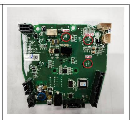
5. Use a fine pair of side cutters to trim down the signal pins. These connections must be trimmed to be as flat as possible so that the spring pin from the plug and play board can make suitable contact with the terminal.
