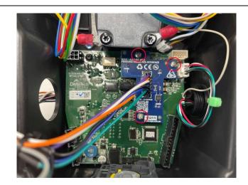
11. Install the Overwatch joystick connectors in series.
