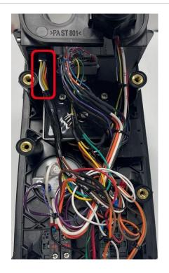
11. Reassemble the control box by suing the 6 bolts taken out earlier and secure the operator sensor cable by using a cable tie.
