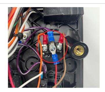
6. Solder the removed original **brown** and **orange** wires to the bare **brown** and **orange** wires from the relay as shown in the image.
