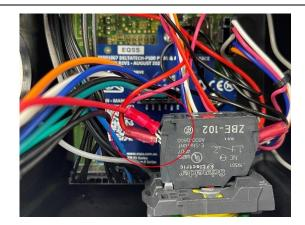
13. Mount the OverWatch ECU inside the joystick control box, the ECU is mounted to the plastic using the adhesive Velcro tape.
