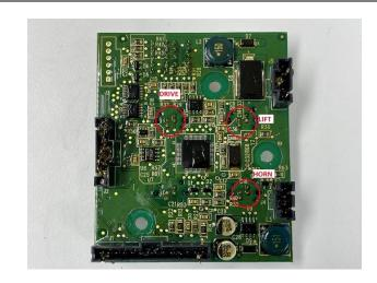
5. Use a fine pair of side cutters to trim down the signal pins.
