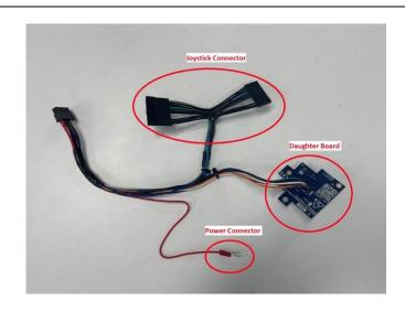
Mount the Overwatch daughter board on top of joystick circuit board.
