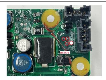
7. Trim down the **Drive** signal pin. This pin is located as displayed in the adjacent image. Using a fine pair of side cutters make sure that the pin is trimmed flat.
