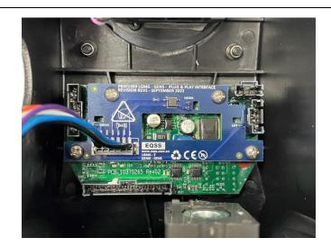
11. Install the Overwatch connectors in between the joystick and the circuit board.
