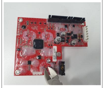
6. Trim down the **Elevate** signal pin as displayed in the image. Using a fine pair of side cutters make sure that the pin is trimmed flat.
