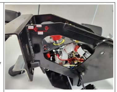
4. Mount the module in the located position using the supplied M4 washers, nuts and security bolts.
