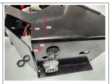
6. Drill a 20mm hole to run the operator sensor M20 Gland into the metal enclosure. The position of the hole is detailed as in the image.
