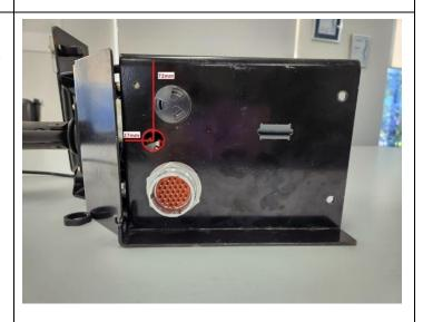
7. Install the supplied cable gland and route the operator sensor cable as shown in the image. Secure the cable to the metal enclosure by using the supplied P-Clips, M4 screws, washers and nuts.
