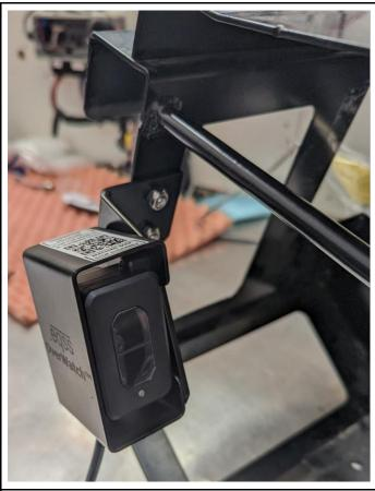
6. Drill a M6 hole at the location shown for the p-clip to secure the operator sensor cable to the control box frame.
