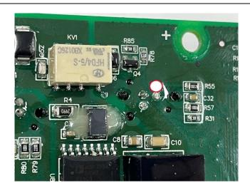
8. Trim down the two **Horn** signal pins. These pins are located as displayed in the adjacent image. Using a fine pair of side cutters make sure that the pins are trimmed flat.
