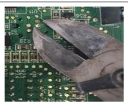
6. Trim down the **Elevate**signal pin. This pin is
