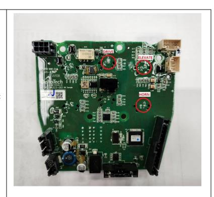
5. Use a fine pair of side cutters to trim down the signal pins. These connections must be trimmed to be as flat as possible so that the spring pin from the plug and play board can make suitable contact with the terminal.
