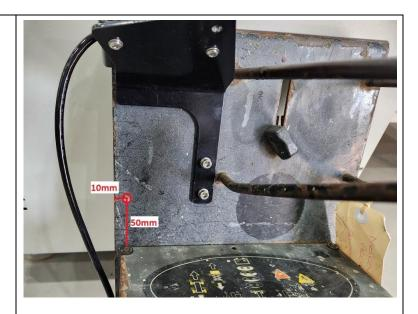
4. Drill two **5mm** holes which are 65mm apart to install the OverWatch ECU. Drill one more **5mm** hole to install another P-clip.
