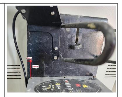
4. Drill two **5mm** holes which are **65mm** apart to install the OverWatch ECU as shown in the image.
