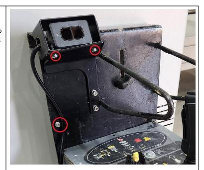
**Note:** Use highlighted holes to position the Operator Sensor.
