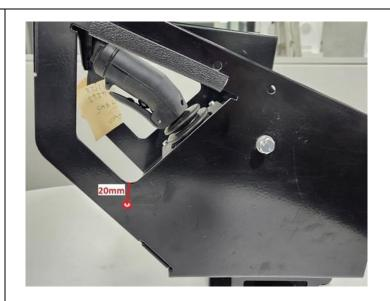
4. Separate the joystick controller from the metal enclosure.
