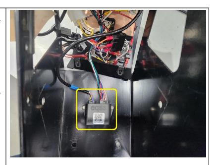
6. Re-assemble the control box. Make sure the operator sensor cable runs clear to the joystick enclosure and tighten the M20 gland to seal the entry point.
