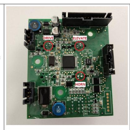
4. Behind the **Drive** select push button, clean, and expose the highlighted pins with a pick.
