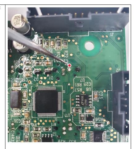
6. Behind the **Horn** push button, clean, and expose the highlighted pins with a pick.
