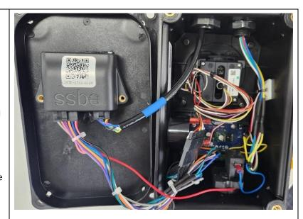
14. Re-assemble the joystick control box and mount to the metal shroud.
