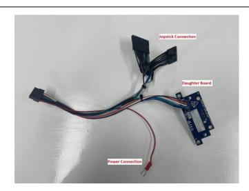
10. Mount the OverWatch daughter board on top of joystick circuit board using the provided screws and spacers in the kit.
