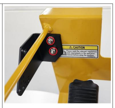
4. Mount the operator sensor in the **45-degree** position on the mounting bracket using the supplied M5 washers and nuts.
