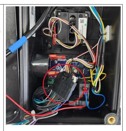
12. At the back of the Estop, install the OverWatch red wire to terminal 2 of the E-Stop.
