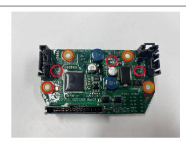
5. Use a fine pair of side cutters to trim down the signal pins. These connections must be trimmed to be as flat as possible so that the spring pin from the plug and play board can make suitable contact with the terminal
