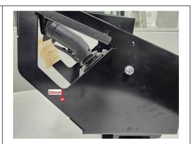
4. Separate the joystick controller from the metal enclosure.
