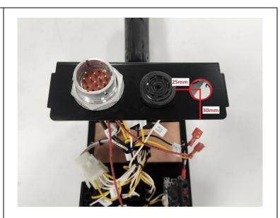
6. Mount the sensor bracket to the control box using M4 nuts, bolts, and washers.
