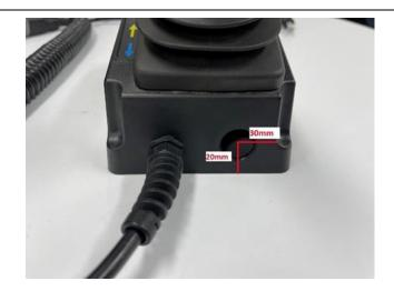
4. Use a fine metal pick to clean the area shown in the red circles, on the adjacent image, to allow access to the pins.
