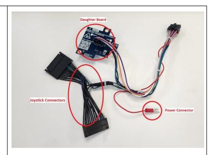
10. Mount the OverWatch daughter board on top of joystick circuit board using the provided screws and spacers in the kit.
