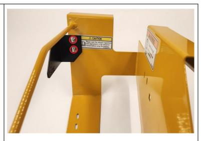
4. Mount the operator sensor in the **45-degree** position on the mounting bracket using the supplied M5 washers and nuts.
