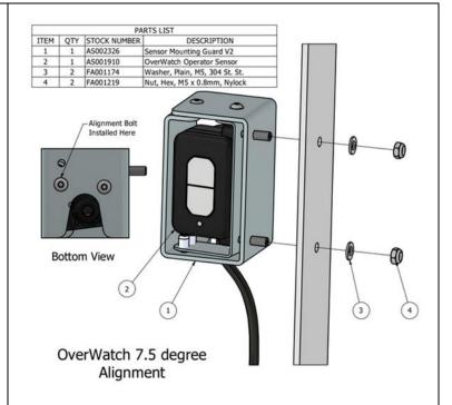
6. Route the operator sensor cable as shown in the image. Use a cable tie to secure the sensor cable to the metal enclosure.
