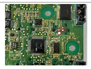
7. Trim down the **Drive** signal pin. This pin is located as displayed in the adjacent image. Using a fine pair of side cutters make sure that the pin is trimmed flat.
