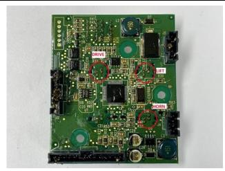
5. Use a fine pair of side cutters to trim down the signal pins. These connections must be trimmed to be as flat as possible so that the spring pin from the plug and play board can make suitable contact with the terminal
