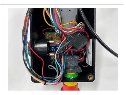
12. At the back of the Estop, install the OverWatch red wire to terminal 2 of the E-Stop.
