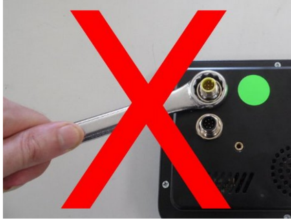
Illustration 7: Do Not Over Tighten Nuts
