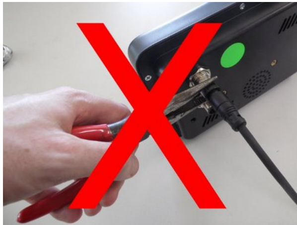
Illustration 6: Do Not Use Tools To Tighten Connector
