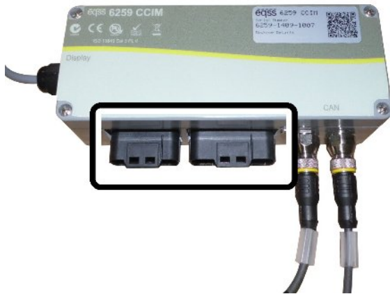
Illustration 1: CCIM Bulkhead Connectors Removed
