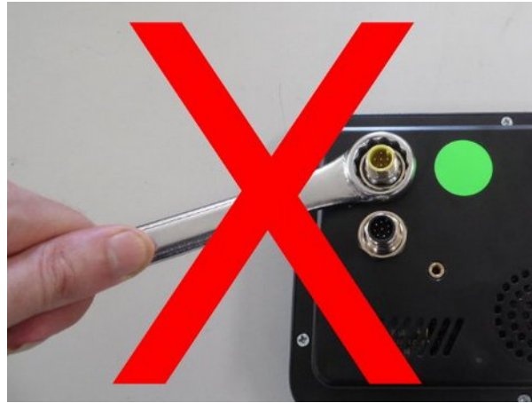
Illustration 9: Do Not Over Tighten Nuts
