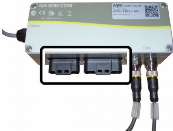
Illustration 1: CCIM Bulkhead Connectors Removed
