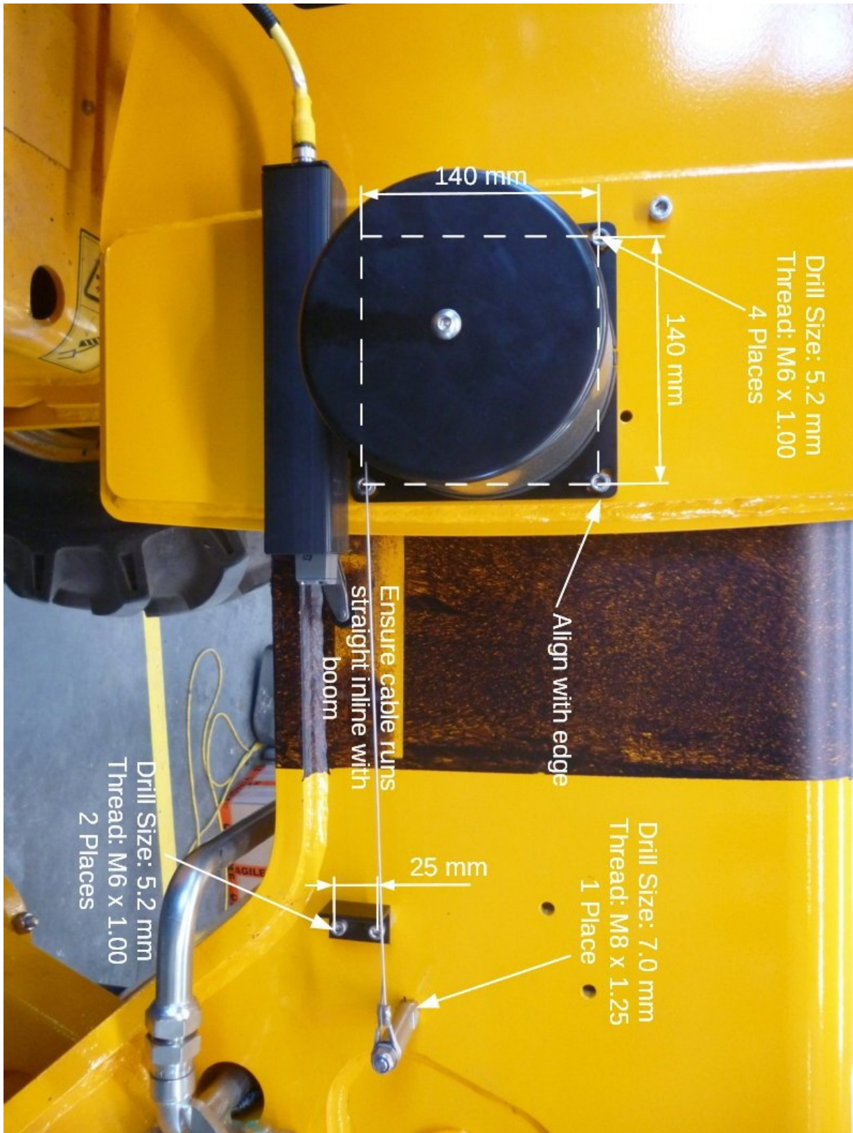
Illustration 1: Cable Reeler Mounting Position
