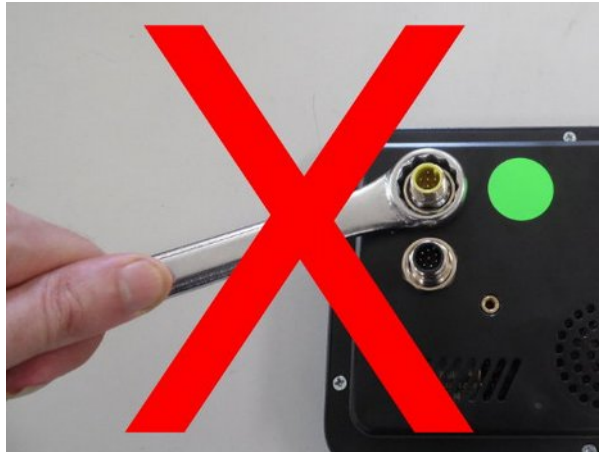
Illustration 7: Do Not Over Tighten Nuts
