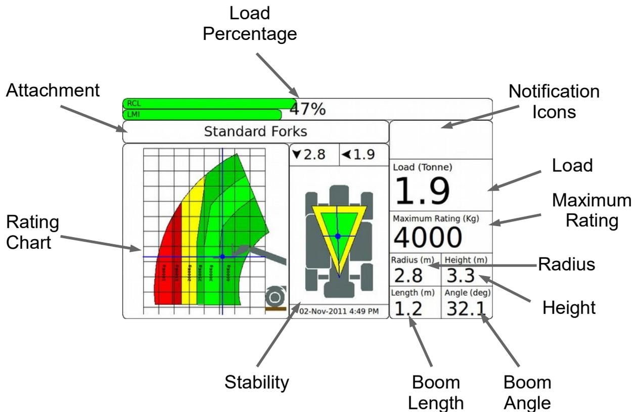
**Load Percentage** – Shows the percentage of maximum load for the Rated Capacity Limiter (RCL) and Load Moment Indicator (LMI). If the LMI has not been fitted there will only be one percentage bar for the RCL. The load percentage number displays the maximum of the two bars. The bars are colour coded depending on their load percentage, with green between 0% - 79%, yellow between 80% - 99% and red 100%+.
