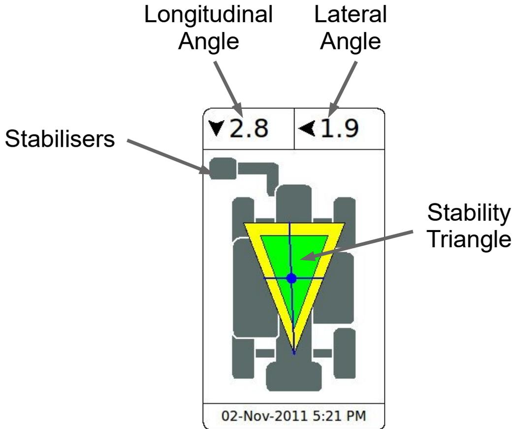
**Longitudinal Angle** – The longitudinal angle shows the current longitudinal angle of the carrier. The arrow indicates the direction of the angle with a down arrow indicating a backward tilt (eg travelling up a hill) and a up arrow indicating a forward tilt (eg, travelling down a hill). The angle is in 0.1 degree increments unless the angle is greater 10 degrees then it is displayed in 1 degree increments.
